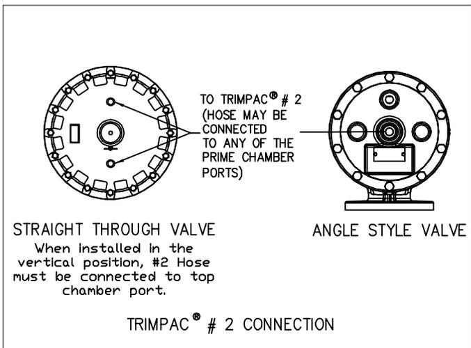
**Figure 11 - Valve Connections**
